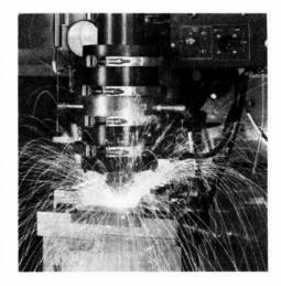
INTERACTION between a laser beam and gaseous metal vapors forms a plasma that permits laser welding, a new capability. Here, 304 stainless steel is being laser welded.
